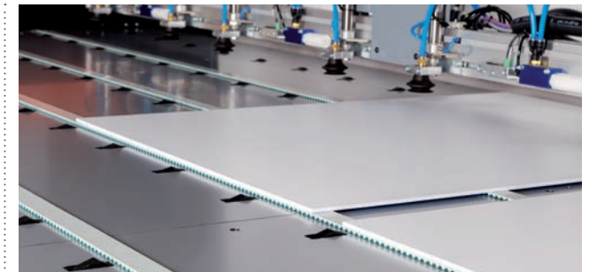
Loads identical or different formats of reams of sheets and panels directly from ground level up to 1.80 meters high.
